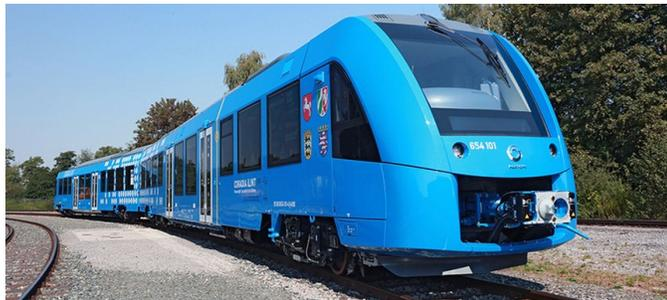
The 300-passenger Coradia iLint regional train uses fuel cell technology to run up to 87 miles per hour. (photo: Alstom)
