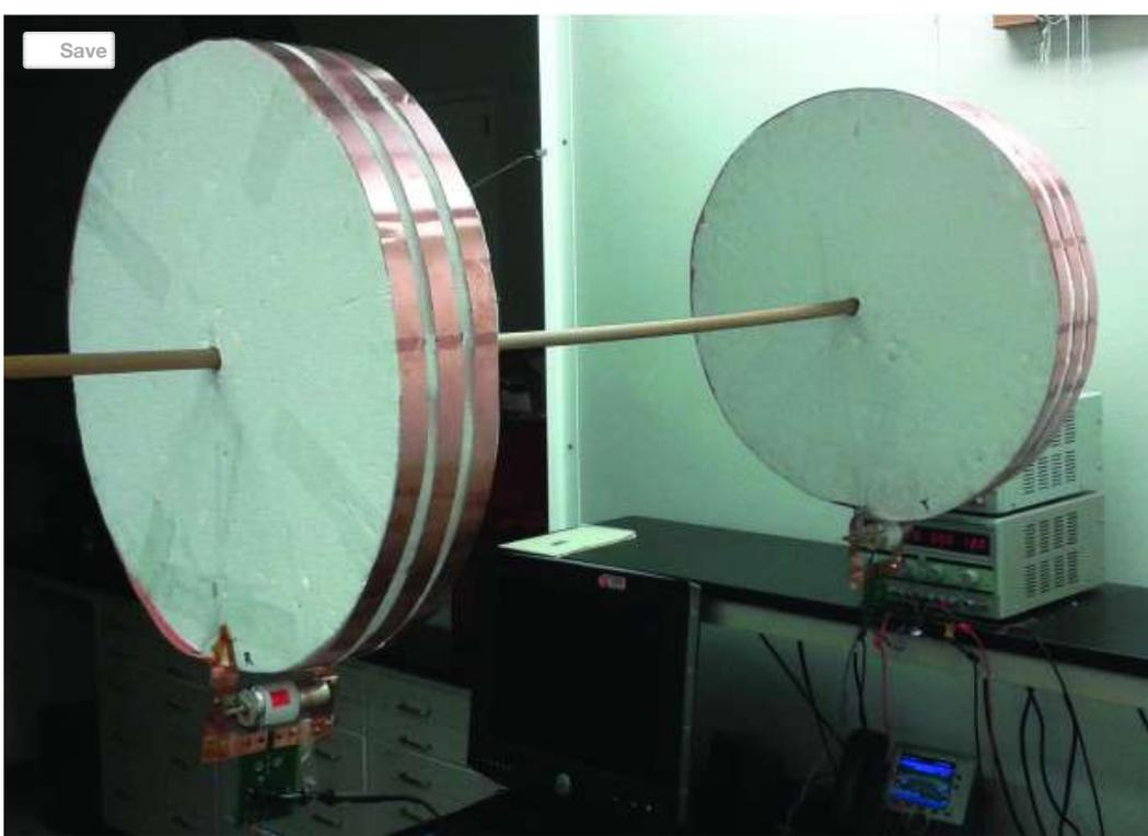
Stanford scientists have created a device that wirelessly transmits electricity to a movable disc. The technology could some day be used to charge moving electric vehicles and personal devices. Credit: Sid Assaworrorarit/Stanford University
